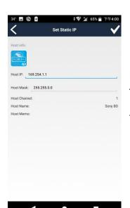
Enter the IP address and subnet mask, then touch top right  $\lceil \mathbf{V} \rfloor$  button to finish settings
