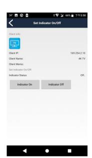
Touch "Indicator On", the ON LED of the host will keep flashing and show an OSD message "I am here" on the monitor Touch "Indicator Off" to stop indicating
