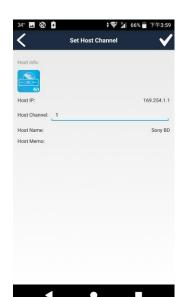
Enter a channel number (0~999) to assign to the host Then touch top right  $\lceil \mathbf{V} \rfloor$  button to finish setting
