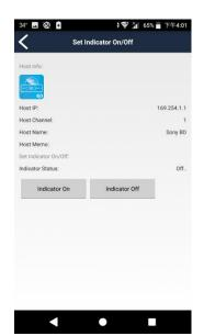
Touch "Indicator On", the "ON" LED of the host will keep flashing
