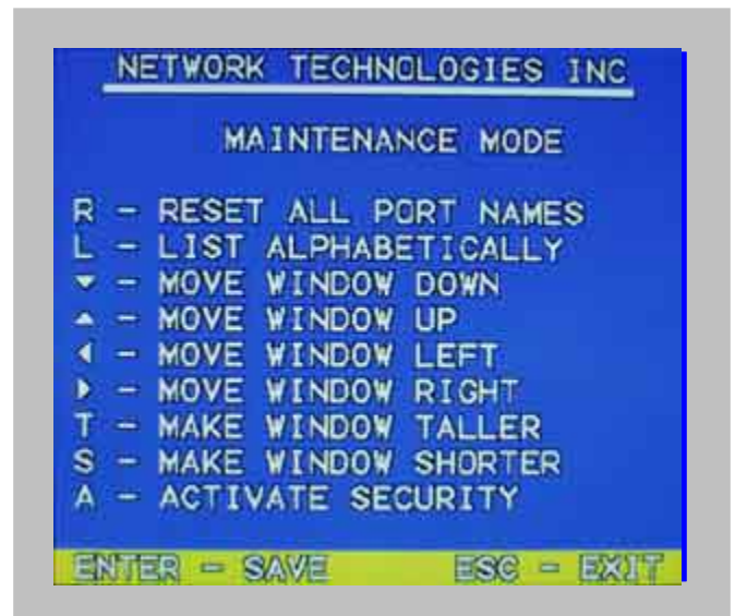
Figure 14- Maintenance Mode screen
